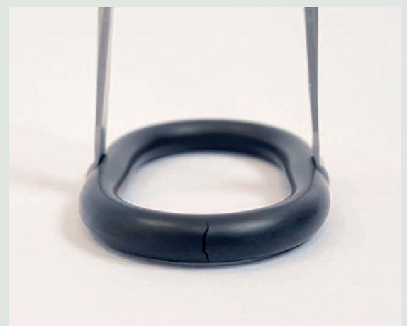
THE DEFECT IS ONLY VISIBLE WHEN THE PIECE IS SQUEEZED
